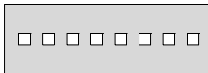
SSR (48 holes/ft.) .5 gpm/in. Minimum nozzle length = 1-1/8"
