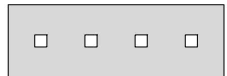
SSR (24 holes/ft.) .25 gpm/in. Minimum nozzle length = 1-1/8"
